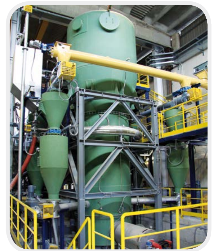
Diagram of operation and image of a fluidised bed Gasifier using EQTEC Gasifier Technology
